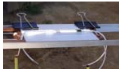
Fig. 3: A single-cell reference PV module based on a triple-junction cell.
