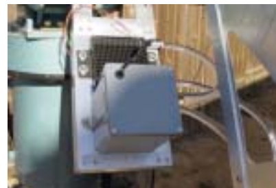
Fig. 4: A water-carrying chiller for reference PV receiver
